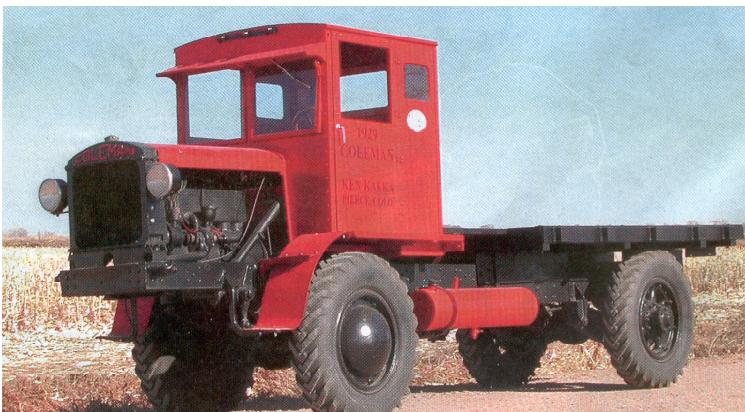
A 1929 Coleman Model DD-40 2 1/2 ton 4 x 4 named "Charlie." Ken Kafka of Pierce Colorado restored it. Charlie is powered by a 400ci Buda BUS engine that puts out 104 hp.
